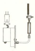
Designed to turn disc electrodes either vertically or horizontally, this accessory serves a dual purpose. When a graphite disc (cat. no. 4011) is placed on the shaft as shown in the upper left photo, the instrument becomes a solution analyzer. Mounted in the lower electrode clamp of the arc stand, as shown in the right-hand photo, the instrument turns a platform electrode.
