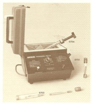
For a troublesome minority of samples, ones that simply can't be ground at room temperature, the Freezer/Mill offers a workable approach. The sample is contained in a vial with magnetic end caps and rod-pestle. The nonmagnetic center section of the vial is submersed in LN<sub>2</sub> while coils at the ends of the vial are energized alternately to attract the rod-pestle back and forth between them. There are as many as 30 impacts per second but without local heating to damage delicate samples.
