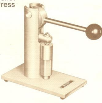
This hand-operated pellet press provides enough force against a small area to prepare, from powder, a suitable tablet for the cup of an electrode. The plunger and die set #3626 produces pellets the proper size for 4005, 4029, and 4030 preforms, while pellets from the #3627 die set fit 4002, 4021, and 4042 preforms.
