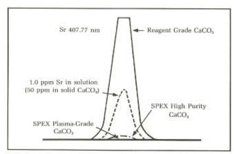
ICP determination of Sr in 2% solutions of CaCO, prepared from reagent grade, high purity and plasma-grade materials. The 1 ppm aqueous Sr solution standard, corresponding to 50 ppm in the solid, indicates the following concentrations of Sr in each material:
