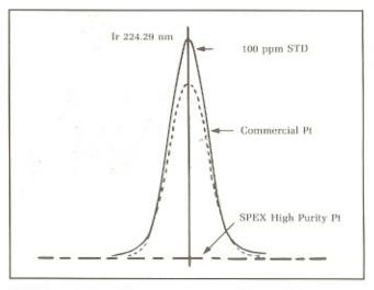
ICP determination of Ir in 1% aqueous solutions of Pt prepared from commercial grade Pt, and SPEX Pt sponge. A solution of 100 ppm of Ir is shown for comparison. The commercial Pt contains around .6% Ir while that in the SPEX compound is undetectable.
