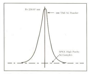
ICP determination of Fe in 5% aqueous solution of Ni prepared from SPEX 4-9s Ni (100 TMI) powder and a specially purified batch of the nickel complex [Ni(NH<sub>3</sub>)<sub>2</sub>](NO<sub>3</sub>)<sub>2</sub>. The concentration of Fe in the 100 TMI sample is estimated at 20 ppm and therefore is less than 1 ppm in the starting material.
