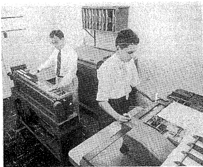
MACHINE MAGIC —IBM machines at Tidewater Oil Company's Delaware Refinery calculate and print out information from the Mass Spectrometer in the refinery's Quality Control Laboratories. Sorter (left) collates the punch cards. Calculating punch (center rear) determines the results. Machine at right prints out final results in visible form.
