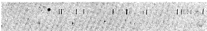
Spectrum taken of Princeton's C Stellarator during pulsing "shake-down". Wavelength interval approximately 250-400A showing many impurity lines of highly ionized carbon and oxygen. Spots on film are typical of the Schumann emulsion used (Eastman SWR).
