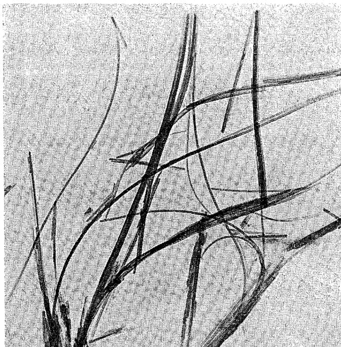
Electron micrograph of chrysotile fibers showing open tubes before grinding.
