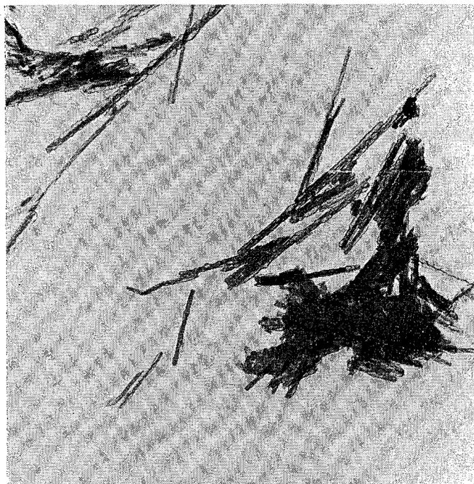
Electron micrograph of chrysotile flattened and broken fibers, after grinding in the Mixer/Mill. High magnification shows individual fibers actually 150-300A in diameter.
