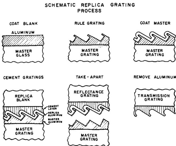
Fig. 4. The replication process for gratings. Here the long face is that blazed. Replication removes the overhanging burr which is seen to intercept a portion of the incoming light to the original. The result is an improvement of efficiency often in the order of 100%. (Courtesy B&L.)
