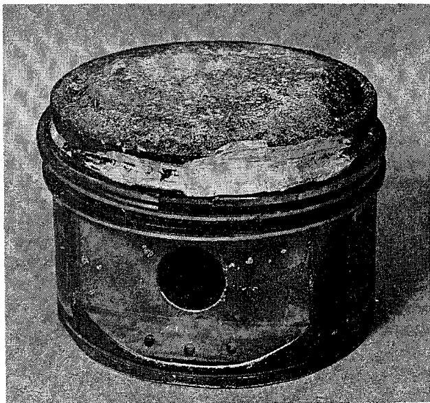
Piston with damaged upper ring land caused by broken ring. Oil analysis indicated high aluminum and iron. (Courtesy NARF)
