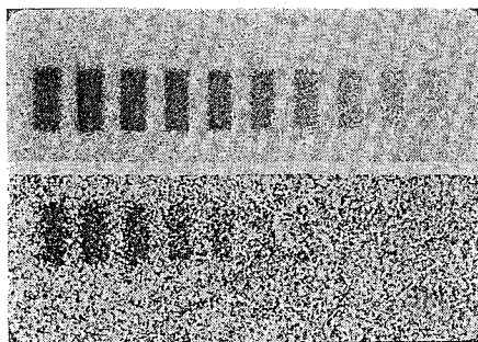
Fig. 2A Identical test patterns were photographed first on a grainy plate then on one considerably less grainy. Despite the fact that the line-to-background ratios are similar, the detectivity of lines in the less grainy emulsion is obviously superior.
