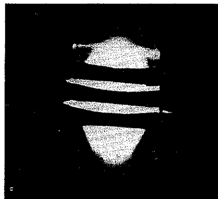
Fig 6 A prolate spheroid plasma is formed when the sample gas and working gas are combined.
