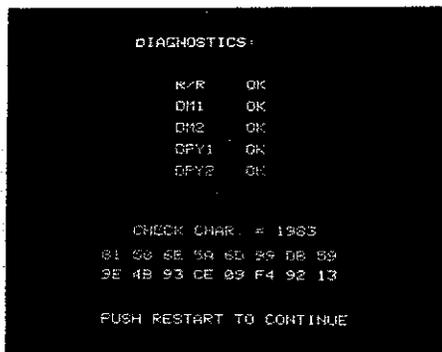
Figure 4 Every time you turn it on, SCAMP reports with a complete diagnostic display. Here the ROM/RAM software, DATA MEMORY, and DISPLAY boards are all OK, and the decimal sum of all 16 PROMS agrees with the check character. If it hadn't, a specific malfunction could be isolated by its hexadecimal code on the bottom of the display.
